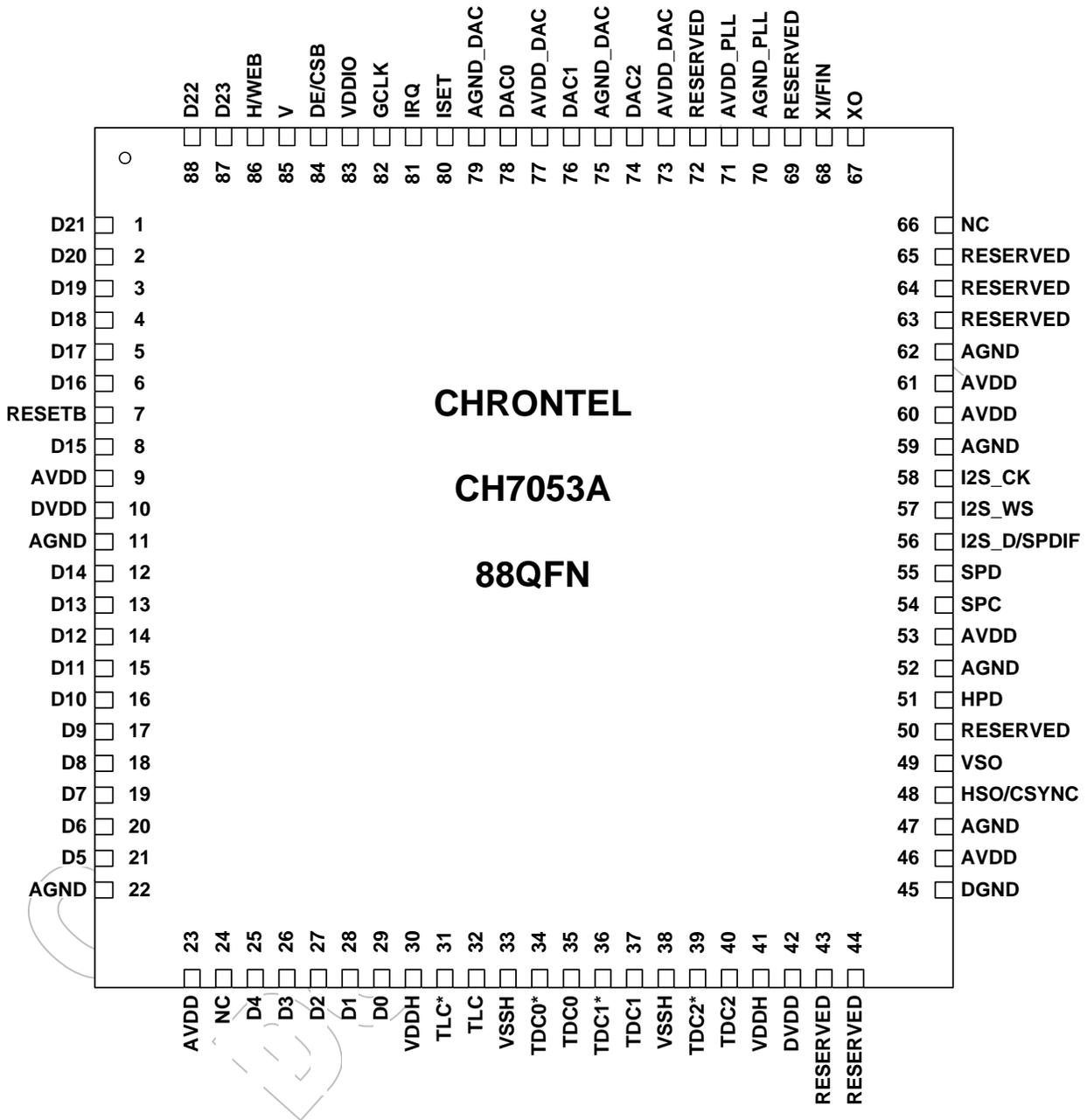
Figure 2: 88 pin QFN Package (Top View)
